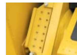
Centralized greasing of the crusher
