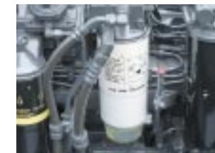
Fuel pre-filter (with water separator)
