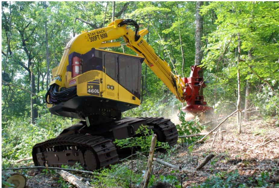
*Komatsu's forest machine with Quadco's felling head*
