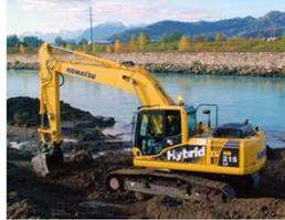
HB215LC hybrid hydraulic excavator operating in Austria
