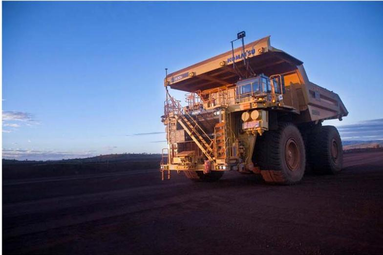
**930E-AT driverless dump truck deployed in Yandi iron ore mine (JSE pit) in the Pilbara region of Western Australia**
