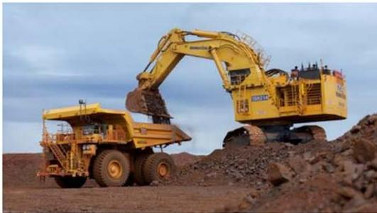
930E-AT AHS dump truck and PC5500 super-large hydraulic excavator
