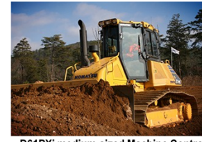
D61PXi medium-sized Machine Control dozer features full automatic blade control.
