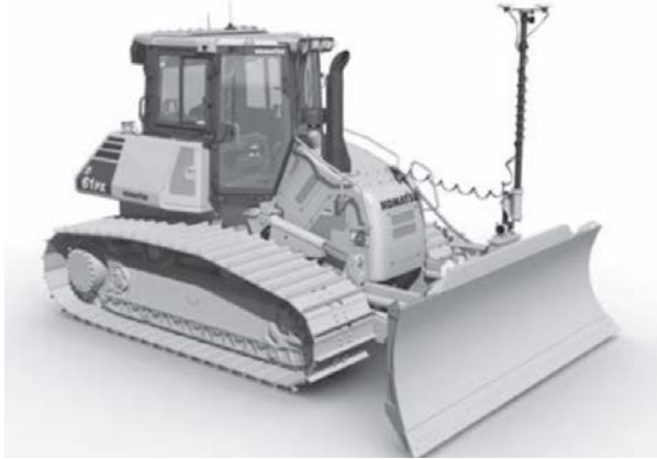
Komatsu D61PX-23 With Typical Aftermarket Machine Control System
