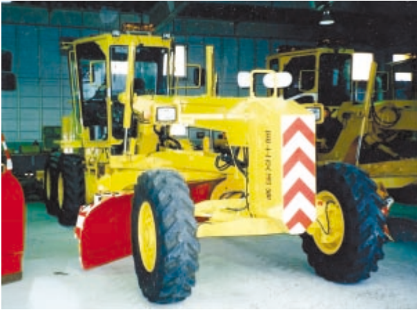
Photo 1 GH320 equipped with combined automatic blade control system
