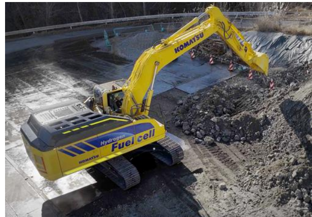
Photo-5 Project A-(1) Excavator FC Excavator Demonstrator equipped with Hydrogen Fuel Cell (example)
