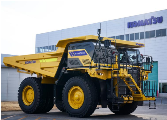
Photo-4 Project A-(1) Concept machine for a large dump truck equipped with a hydrogen engine (example)
