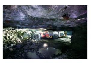
[GHH's load haul dump suitable for narrow tunnels]
