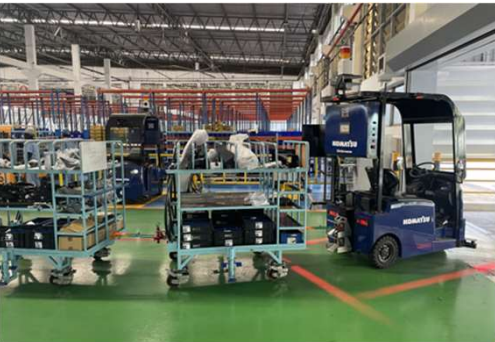
Unattended transport of parts using AMR in the Thai Plant
