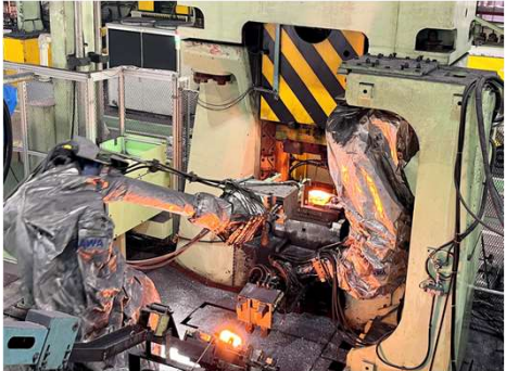
Automated hammer forging process
