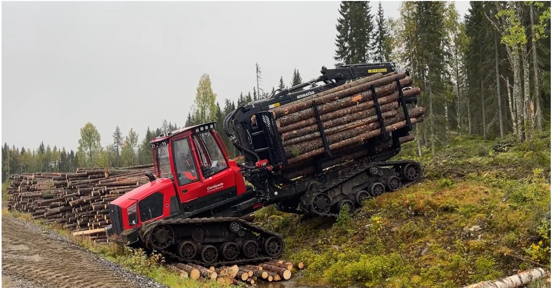
【Photo】 Soil-friendly crawler-type forwarder, Centipede (Concept machine)
