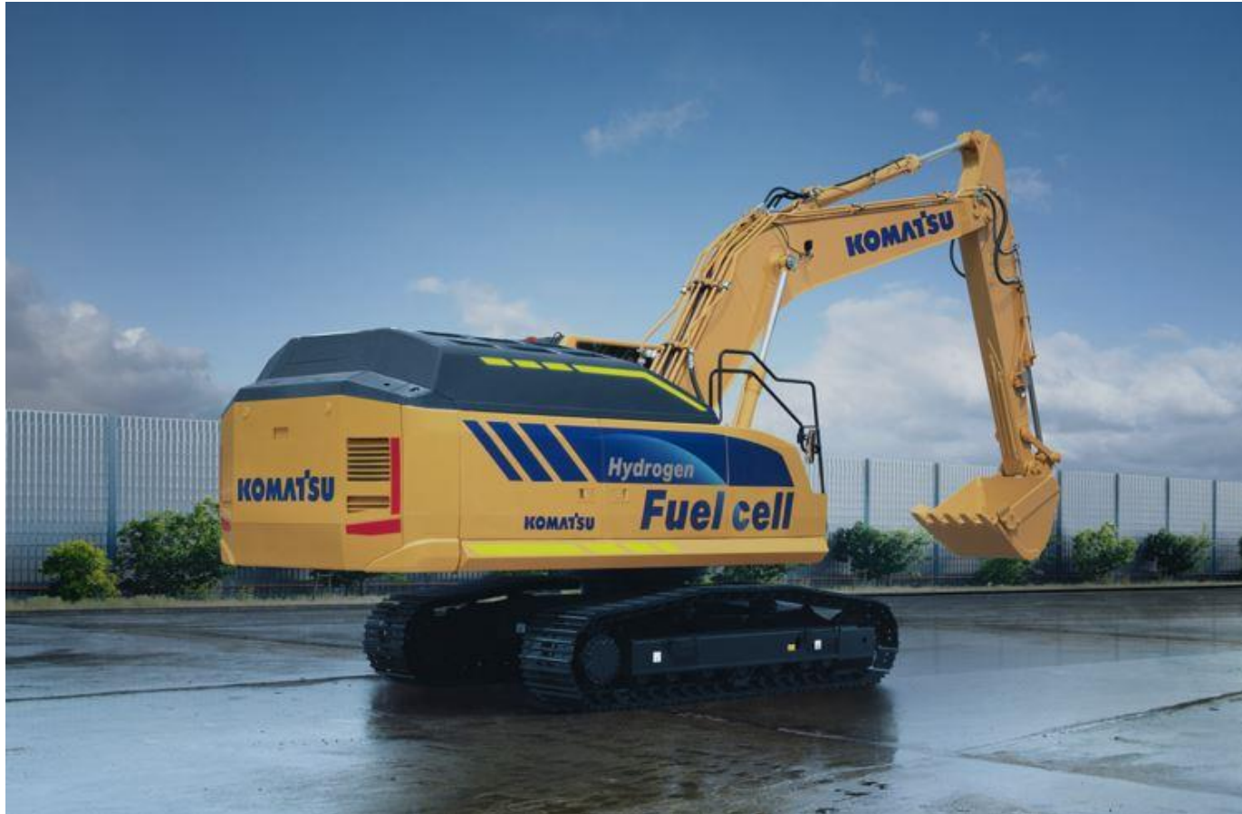
【Picture】 medium-sized hydraulic excavator equipped with hydrogen fuel cell (concept machine)
