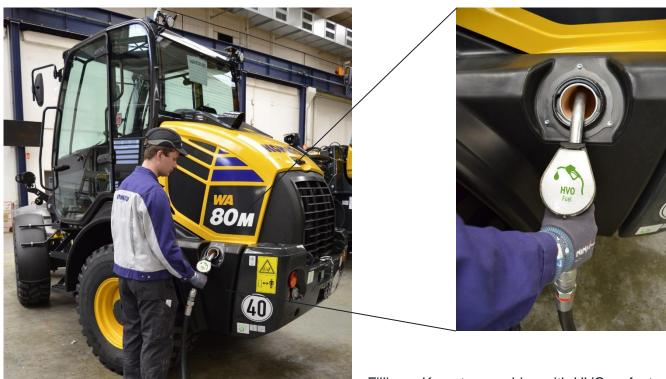
Filling a Komatsu machine with HVO as factory-fill fuel at the KGC plant in Hannover, Germany
