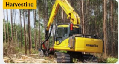
PC130F Harvester (forest machine based on hydraulic excavators)
