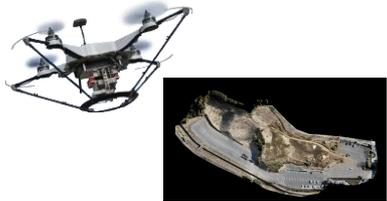
High-precision 3D survey by using drones
