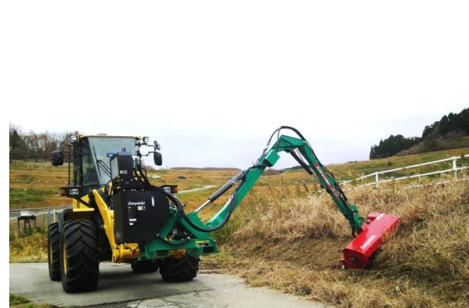
Weeding and soil transportation by using multifunctional wheel loader (Regeneration of farmland and labor-saving)
