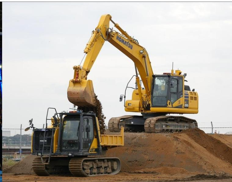
Autonomous hydraulic excavator and crawler dump working together
