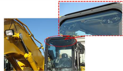
Stereo camera installed on a PC200i Machine Control hydraulic excavator
