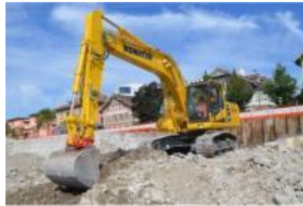
Hydraulic excavator (Crawler-type)
