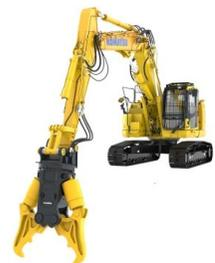
Hydraulic excavators (with pulverizer)
