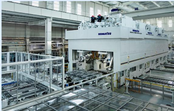
Large size AC servo press system [Komatsu Industries Corp.]
