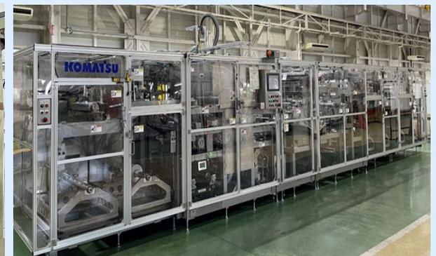
Manufacturing equipment for vehicle batteries [Komatsu NTC Ltd.]
