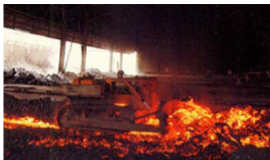
Radio-controlled bulldozer used for slag handling at a steelworks (D125AR)
