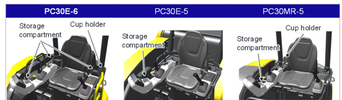
Fig. 18 Addition of storage compartment
