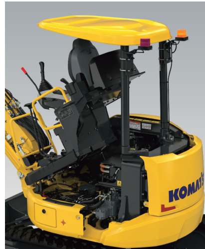
Fig. 12 Tilt-up mechanism (from the photograph in the catalog)
