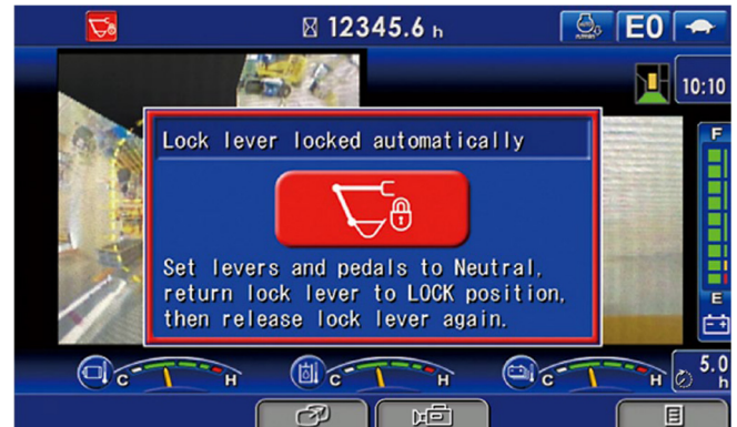
Fig. 11 Monitor display when the lock lever auto-locking function in operation
