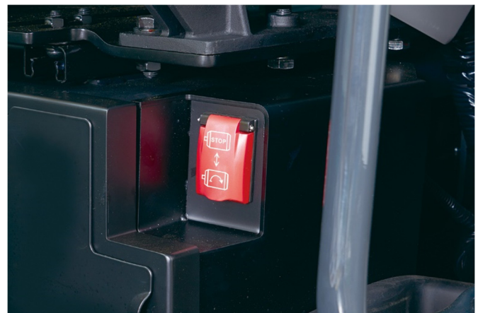
Fig. 12 Motor stop secondary switch
