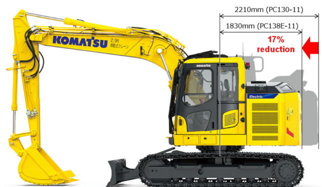
Fig. 6 Tail swing radius of PC138E-11
