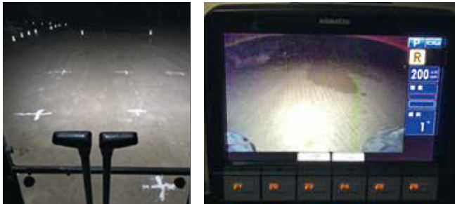
Fig. 4 Night visibility - front (left) / rear monitor camera (right)
