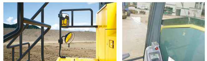
Fig. 2 Right-side visibility from the operator's seat - developed model (left) vs. conventional model (right)
