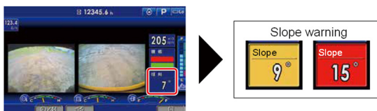
Fig. 5 Digital display of inclination angle
