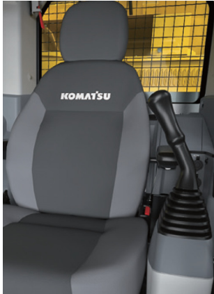
Fig. 18 Body and swing combined operation control lever
