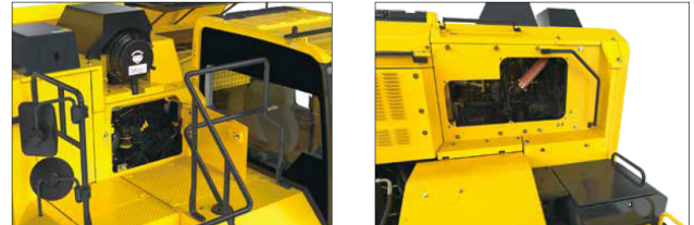
Fig. 11 Engine room front and rear maintenance space
