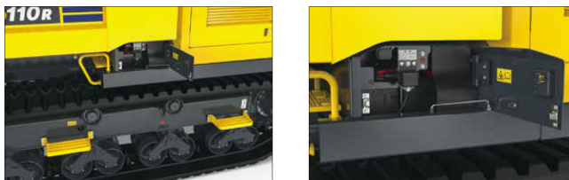
Fig. 14 Battery access and battery disconnect switch
