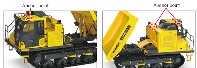
Fig. 7 Machine tie off anchor points and improved ability to go up and down
