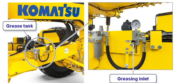
Fig. 14 Auto-greasing tank and greasing inlet (on the work equipment)
