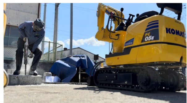
Fig. 7 Example of using hydraulic outlets for attachments: Breaker
