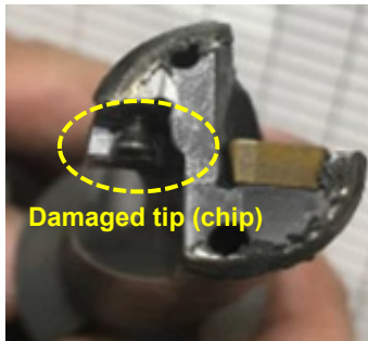
Fig. 4 Damaged cutting edge of a tool (chip)
