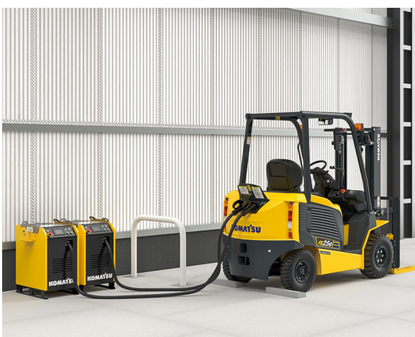
Fig. 8 FE25G-2 fast charging with a dual fast charger (Source: Brochure)
