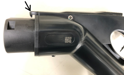
Fig. 13 Locking device on the plug
