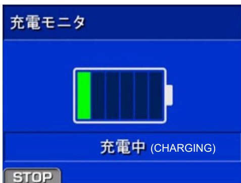
Fig. 12 Automatic charge start display on the vehicle monitor panel
