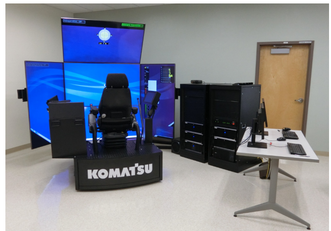
Fig. 4 Teleoperation station (Entire view)
