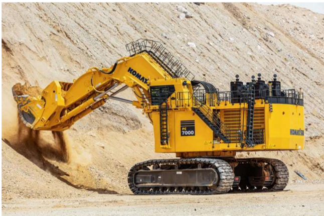
Fig. 3 PC7000-11 retrofitted with a teleoperation kit
