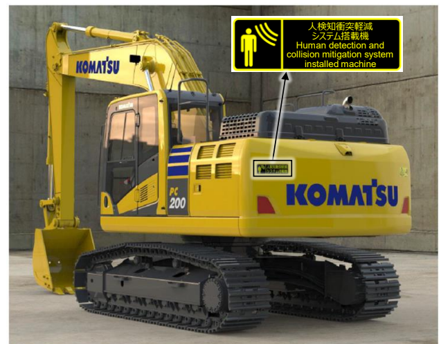
Fig. 4 External appearance of PC200-11 fitted with KomVision human detection and collision mitigation system (a decal is added)
