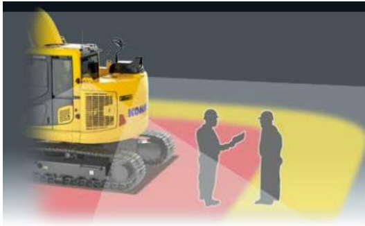
Fig. 16 Application of human detection and collision mitigation system on PC138US-11
