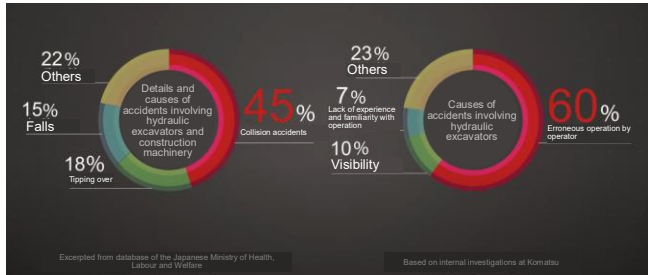
Fig. 2 Details and causes of accidents involving hydraulic excavators and construction machinery
