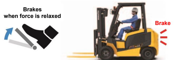
Fig. 16 Accelerator one-pedal mode
