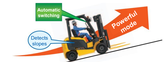
Fig. 7 Automatic switching of power mode for uphill travel
