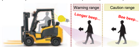
Fig. 15 Overview of collision detection alarm system
