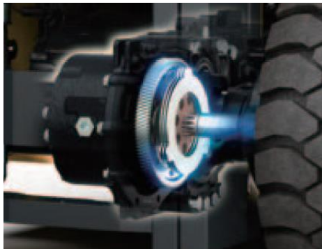
Fig. 2 Sealed wet type multiple disc brake
