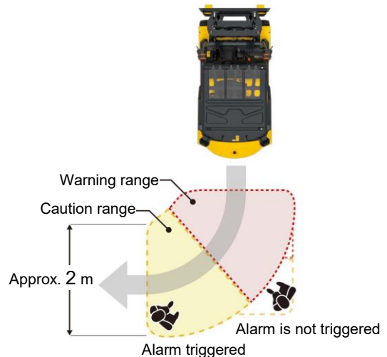
Fig. 13 Alarm range when vehicle is reversing (and turning) (excerpted from Safety Booklet)
