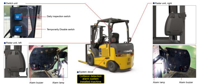
Fig. 3 External appearance of collision detection alarm system (FE25/25H/30-1) (excerpted from Safety Booklet)
