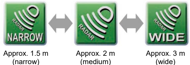
Fig. 14 Alarm range width (variable in three stages only with FE25/30-2) (excerpted from Safety Booklet)
