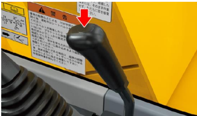
Fig. 11 Travel changeover switch added to the blade control lever
