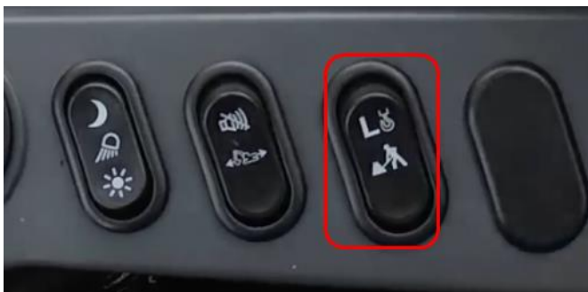
Fig. 12 Arm crane one-touch changeover switch
