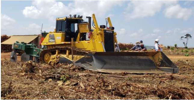
Fig. 3 D155EX-6 modified as a subsoiling version
