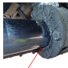
Fig. 6 Oil leak due to rod damage
