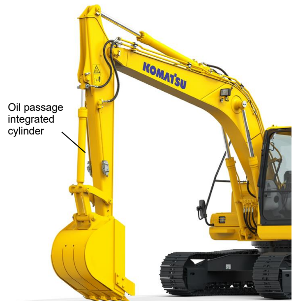
Fig. 1 PC130-10M0 oil passage integrated cylinder installed vehicle
