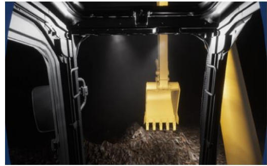
Fig. 13 Example of night visibility evaluation simulation
