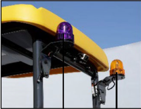
Motor-in-operation beacon lamp Beacon lamp for arm crane
