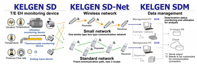
Fig. 14 Overview of the KELGEN SD system
