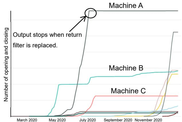
Fig. 9 Number of opening and closing of bypass valve of each machine
