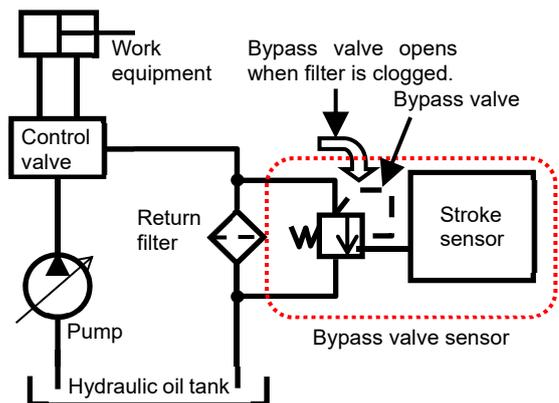
**Fig. 1** Simple circuit diagram of construction machinery filtration system
