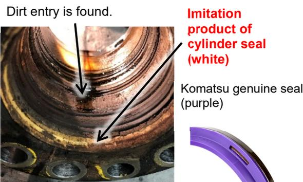
Fig. 11 Photo inside the cylinder which uses an imitation product
