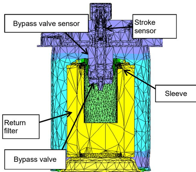
Fig. 7 Deformation of bypass valve sensor by pressure
