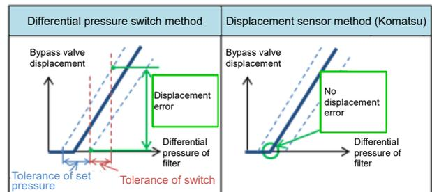
Fig. 4 Effect of detecting methods of bypass valve sensor on error
