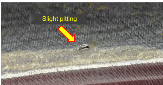
Fig. 5 Tooth surface after durability test operation
