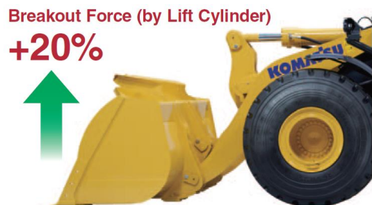
Fig. 5 Improved breakout force by lift cylinder
