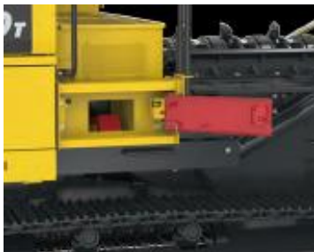
Fig. 19 Boarding prevention gate
