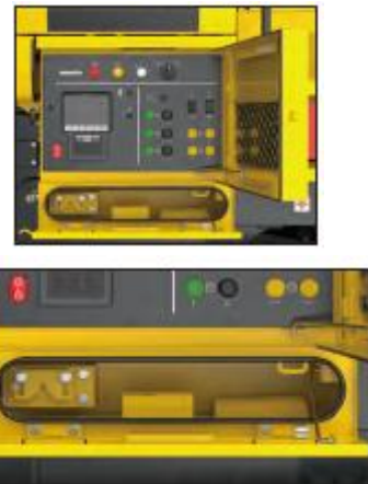
Fig. 13 Radio control storage space
