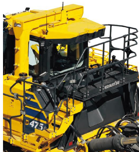
Fig. 7 Platform for maintenance facing two surfaces
