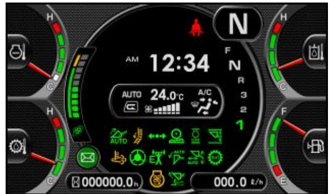
Fig. 18 Machine monitor with 7-inch high definition LCD unit
