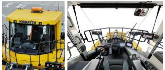
Fig. 10 Large cab with a trainer seat
