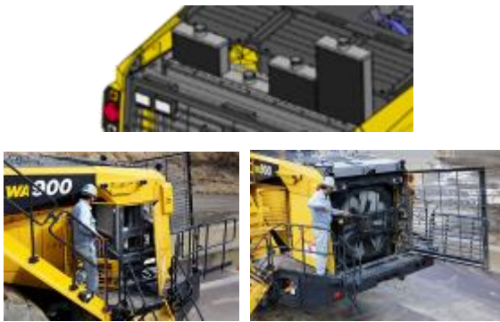
Fig. 16 Radiator core maintenance
