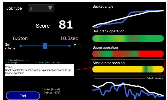
Fig. 14 Operation guidance monitor display
