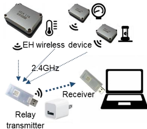
Fig. 13 Example of configuration of the on-premise system
