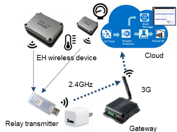
Fig. 14 Example of configuration of the cloud system
