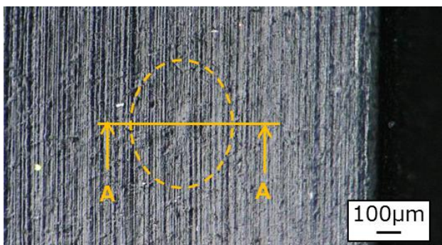
Fig. 3 Oil seal lip surface after testing
