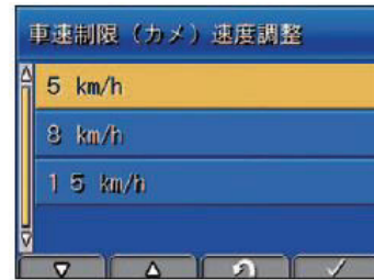
Fig. 10 Travel speed limit setting screen
