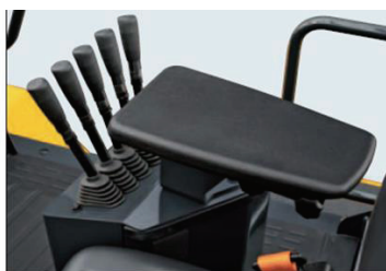
Fig. 9 Levers and large arm rest for controlling the work equipment at the hand position
