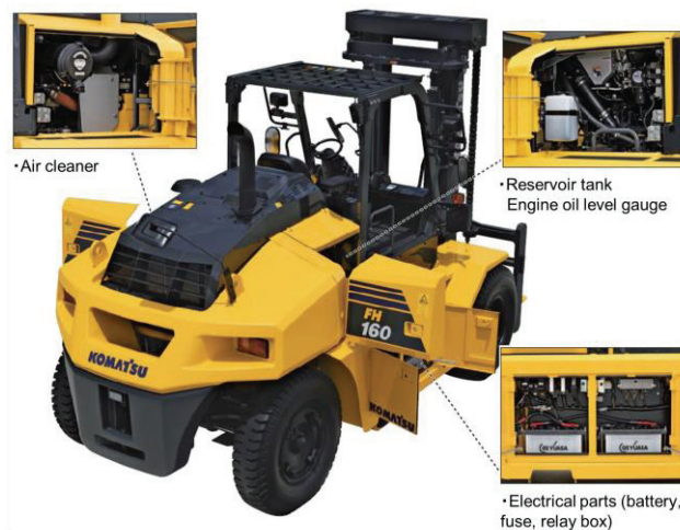
Fig. 15 Large inspection cover
