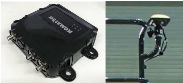
Fig. 14 GNSS Surveying Equipment
