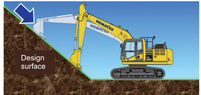
Fig. 5 Bucket Angle Hold Control
