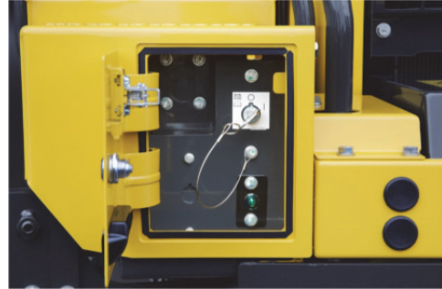
Fig. 16 Battery disconnect switch
