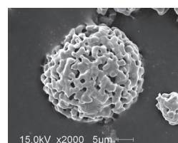
Fig. 7 Appearance of a particle to be thermal-sprayed
