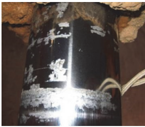
Fig. 2 Rusting of a cylinder rod
