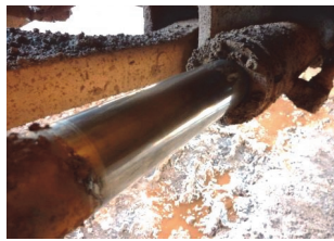
Fig. 3 HVOF thermal-sprayed cylinder rod
